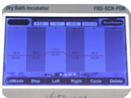
Figure 6. The PIPseq™ Dry bath to be used for the lysis incubation step.
