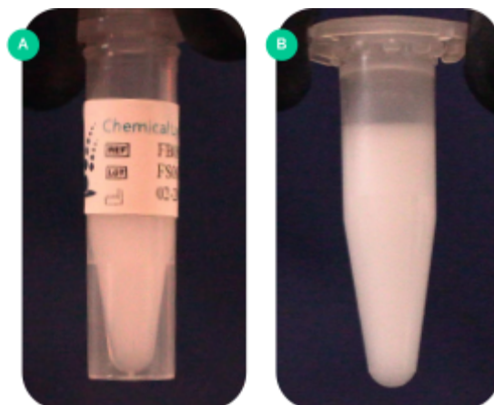
Figure 5. Chemical Lysis Emulsion after addition of Partitioning Reagent and vortexing (A). Sample tube after addition of Chemical Lysis Emulsion and inverting (B).
