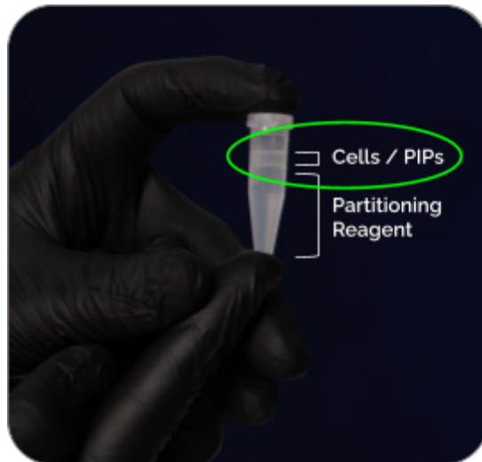
Figure 1. (circled in green) Cells and PIPs mixture floating on top of excess Partitioning Reagent
