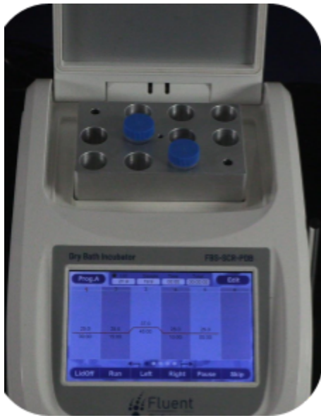
Figure 6. The PIPseq™ Dry bath to be used for the lysis incubation step.
