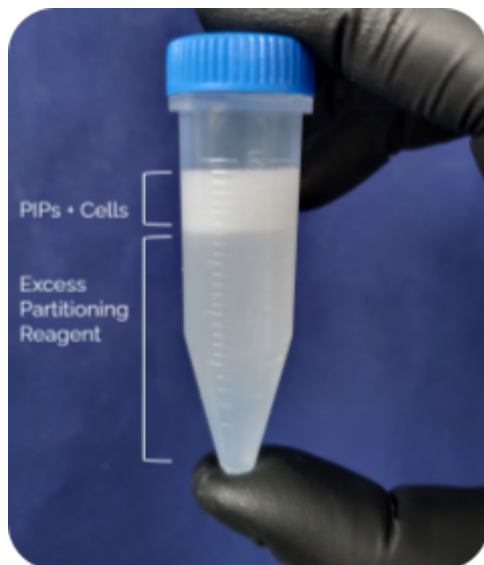
Figure 3. Emulsified PIPs and cells are seen floating in the top phase while the excess Partitioning Reagent in the bottom phase.
