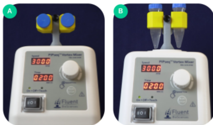
Figure 2. The rotating vortex adaptor shown in the horizontal configuration (A) and the vertical configuration (B).
